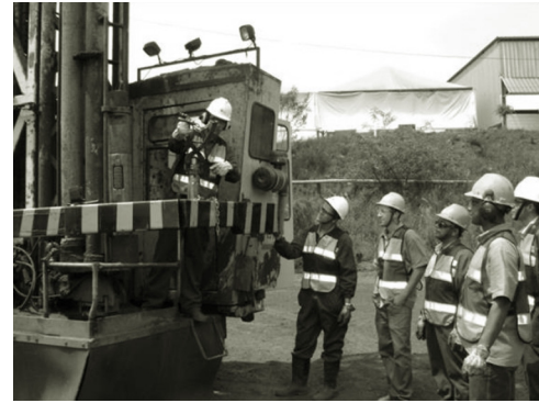
Fig. 5 – Bit replacement device in operation.
